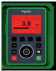
Detected fault: Red screen when there is a detected error
