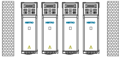
a. Unlimited left and right space (no communication expansion board)
