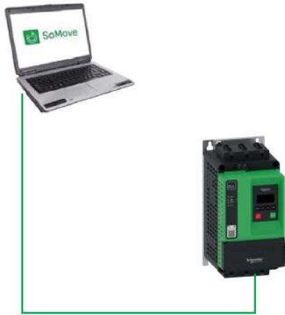
Firmware update through Modbus serial using SoMove
