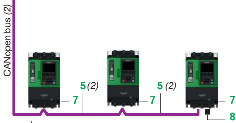
Altivar Soft Starter ATS490 + VW3A3628 module Example of connection to the CANopen bus with a screw terminal block
