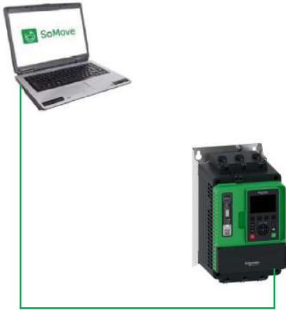
Firmware update through Modbus TCP/Ethernet/IP or Modbus serial using SoMove
